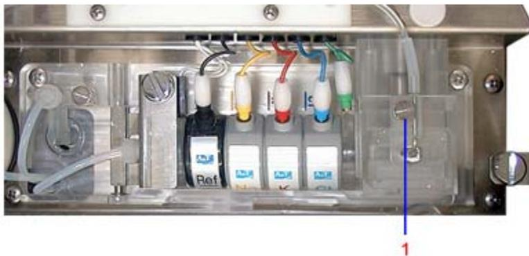
**Figure 5-39. Location of the liquid-supply nozzle**
