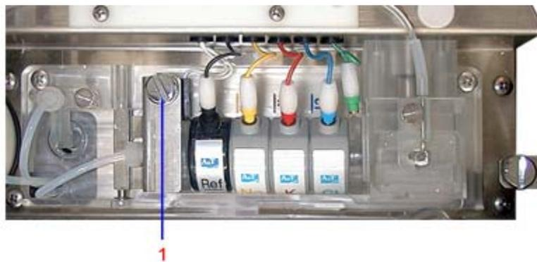
Figure 5-37. ISE electrode plate thumbscrew
