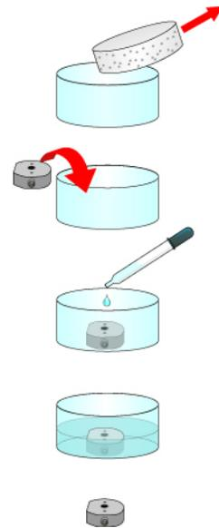
Figure 5-38. Soaking the electrode
