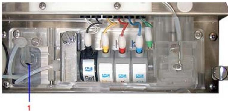
**Figure 5-40. Location of waste-drain nozzle**
