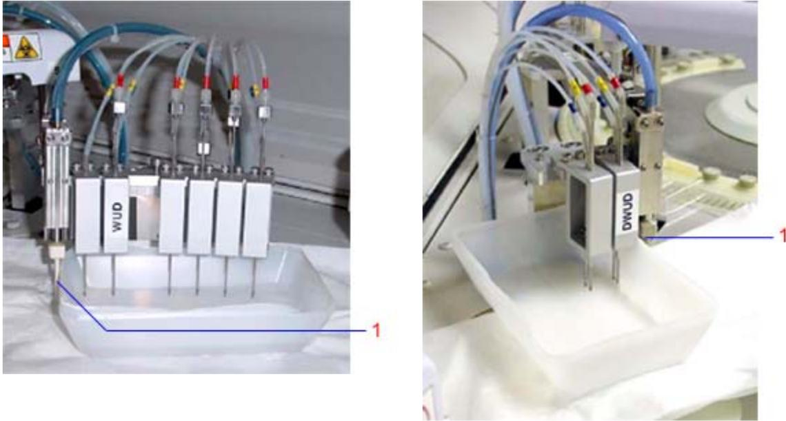
**Figure 5-35. WUD and DWUD dryer nozzle**
