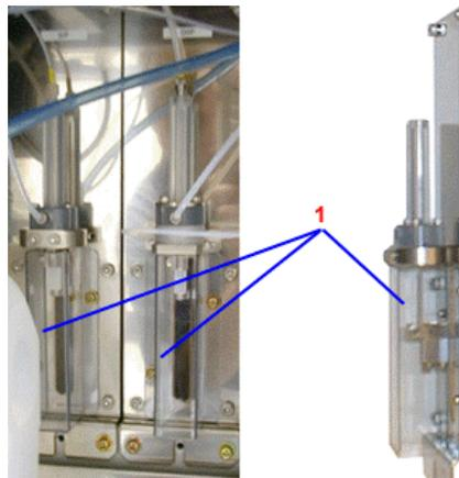
Figure 5-10 Sp and DIP vertical pumps
