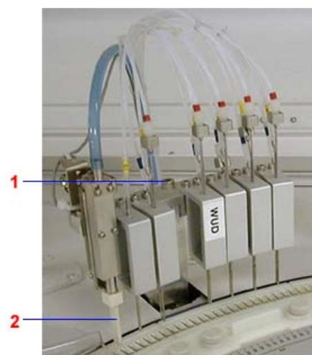
Reaction cuvette wash station (WUD)
