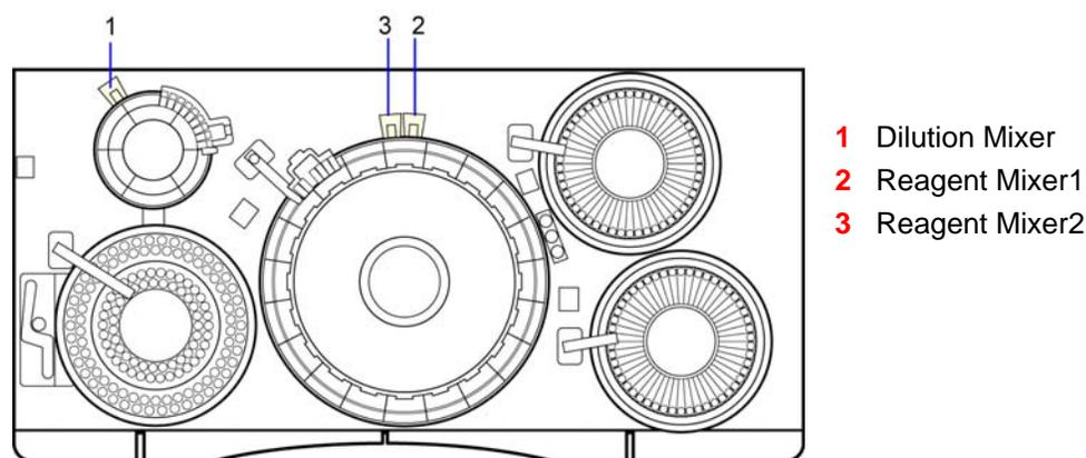
**Figure 5-3. Mixing rods**
