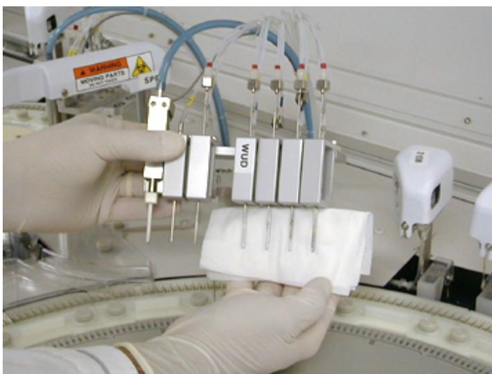
**Figure 5-6. Wiping the wash stations with lint-free towels**
